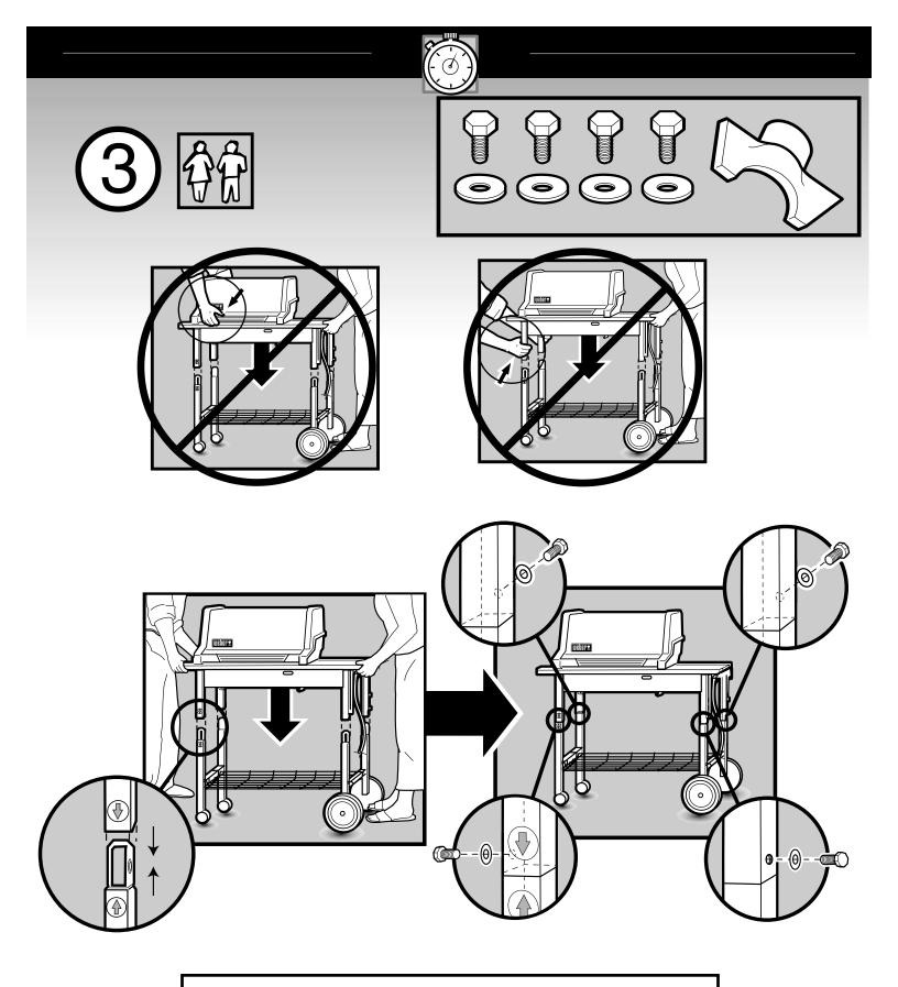
• Install bolts at indicated locations. Use supplied tool to tighten. Recheck each bolt for tightness with a 7/16" open end wrench.
